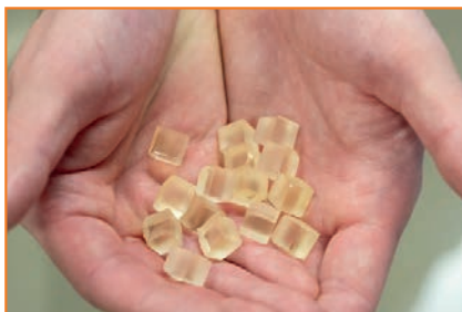
Photo shows small cubes of the PolyEster Covalently Adaptable Network (PECAN) resin. (Photo by Werner Slocum/NREL)
